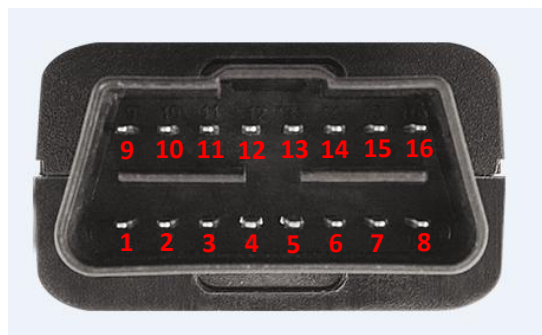
Figure 2. OBD II Connector on GV500MAP
