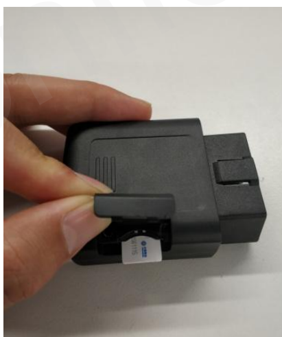
Figure 6. SIM Card Installation
