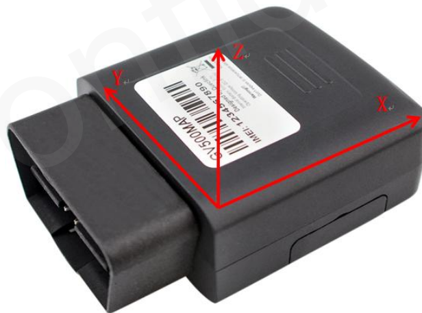
Figure 3. Motion Sensor Direction
