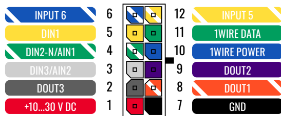
FMC130 2x6 socket pinout
