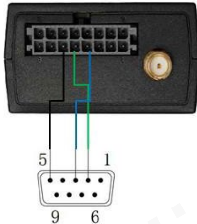
Figure 16: Connection with RS232 Port
