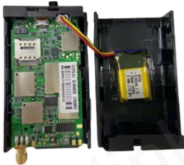
Figure 6: Backup Battery Installation
