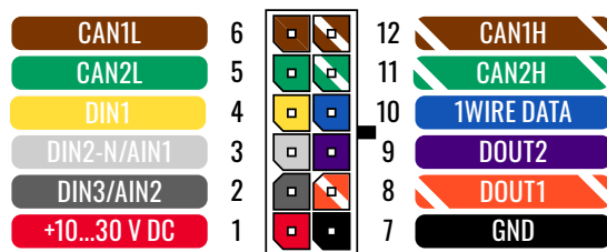
FMB140 2x6 socket pinout
