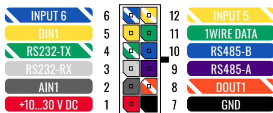
FMB125 2x6 socket pinout
