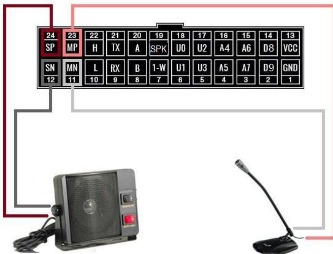
Figure 9 – Diagram of connecting the microphone and speaker
