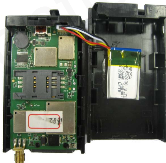
Figure 6. Backup Battery Installation
