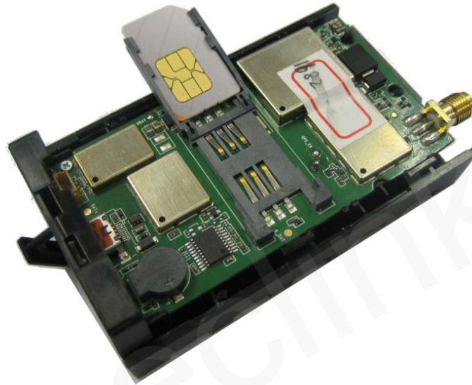
Figure 5. SIM Card Installation
